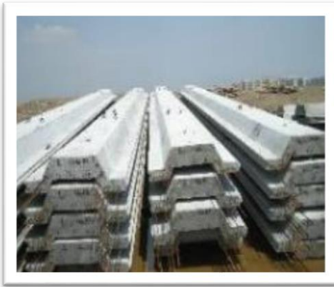
RETAINING WALL CONCRETE
